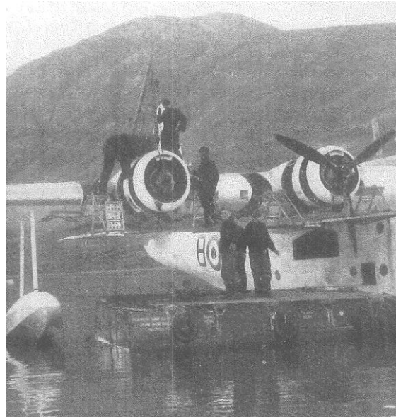
A Magnificent Job Engine swap under difficult conditions
